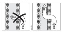
If the exhaust air is to be ducted into a vent flue, the ducting must be directed in the flow direction of the flue
